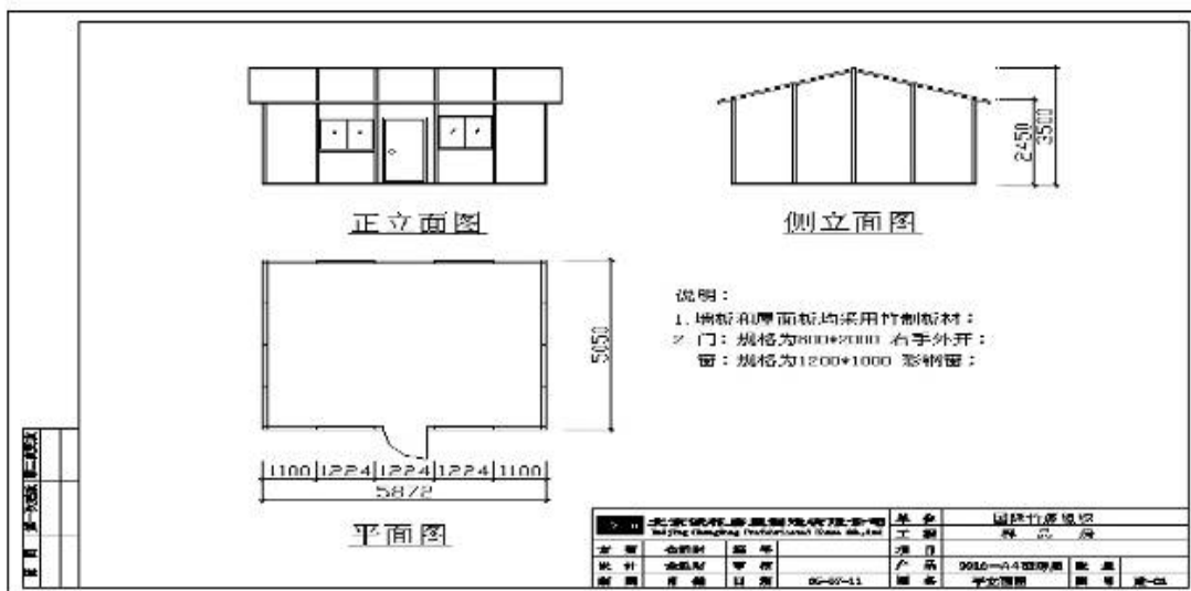
Fig.2 Demonstration bamboo panel prefabricated house
