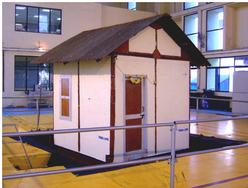
Figure 2: Bamboo house mounted on seismic table for testing
