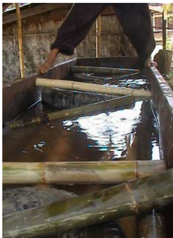
Bamboo in preservation tank (the culm pieces across the tank help keep the culms submerged)
