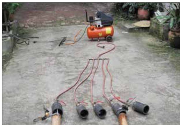
Figure 24: Modified boucherie treatment plant
