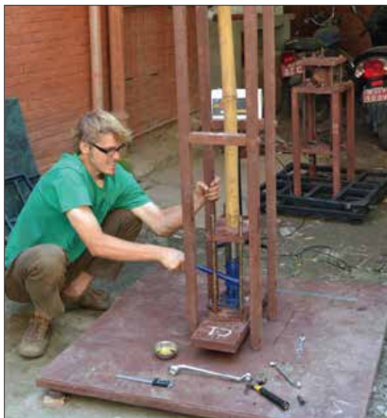
Figure 18: INBAR-developed portable strength grading test kit
