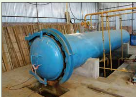
Figure 28: Bamboo pressure chamber treatment unit
