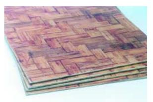
Fig. 2-29: The appearance of woven-mat plybamboo
