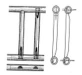
Fig. 3-47 Oblique dowel joint
