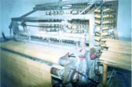
Fig. 3-4: Bamboo-mat weaving machine
