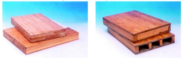
a. Solid bamboo strip-wood panel. **Fig. 2-43: The outward appearance of bamboo strip-wood panels**
