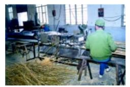
Fig. 3-3: cut into bamboo threads on a threading machine
