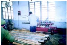
Fig. 3-1a: Bamboo splitting machine
