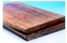
Fig. 2-34: The appearance of glued sliver plybamboo
