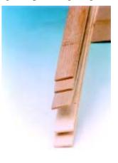
a. Pressed and flattened. b. Planed. Fig.1-20. Bamboo strips made in different ways
