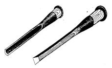
Fig. 3-21 Gouge and square chisel
