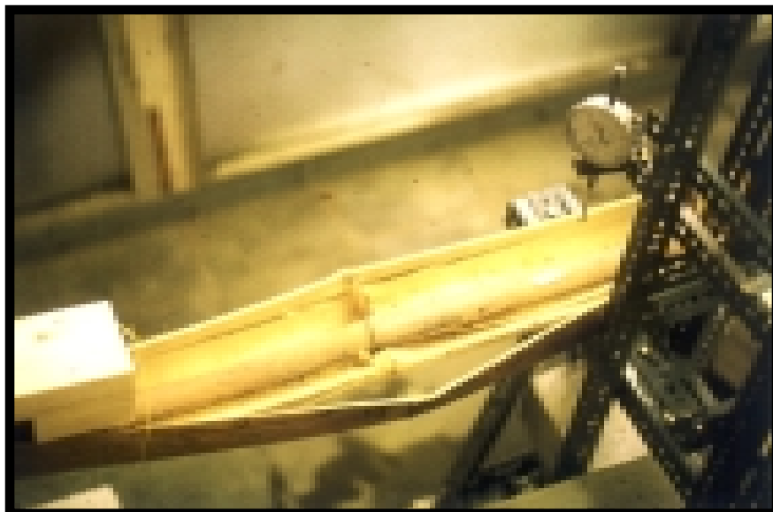
Fig. 14: Failure in bending for bamboo (Technical University of Eindhoven)
