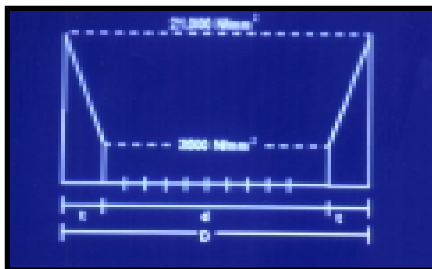
Fig. 45: E-modulus in culm wall
