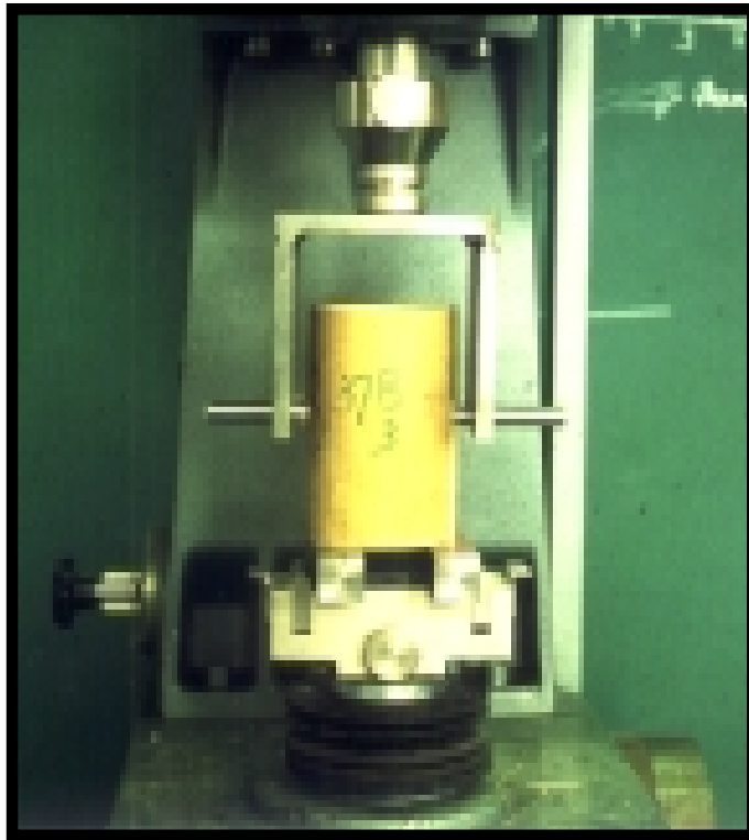
Fig. 46: Test on shear with bolt in bamboo
