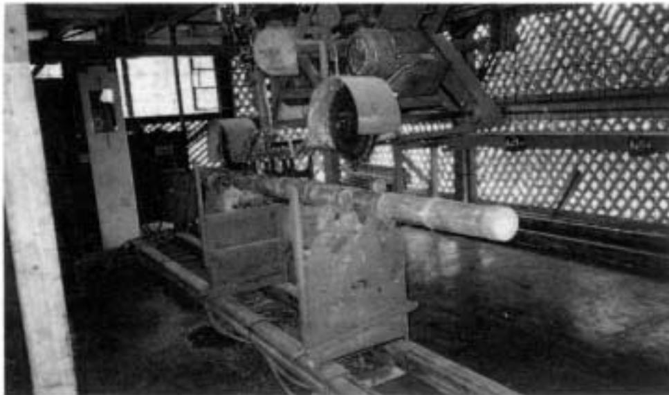
Fig. 11: Cutting bamboo culm into tabi//a, at CITAB, Milan0
