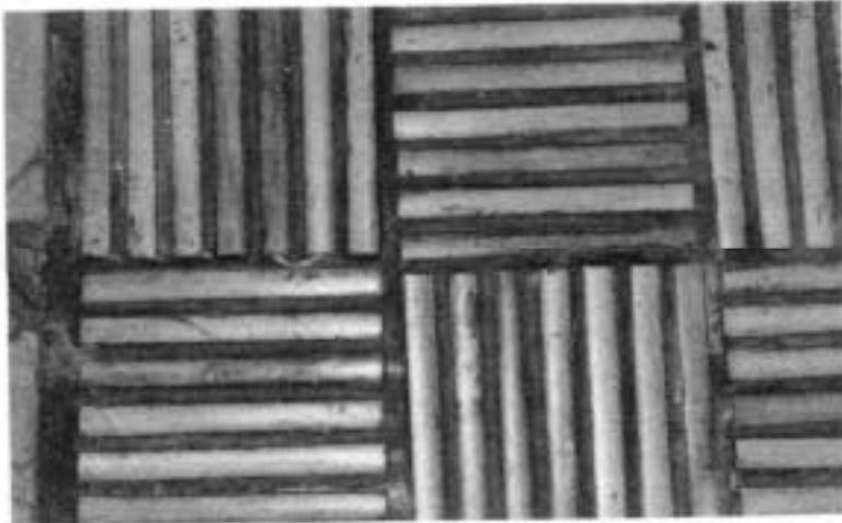
Fig. 24: Bamboo parquet flooring being developed at CITAB, Milano
