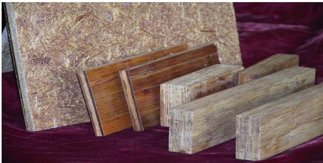
Fig. 1 the panels laminated along the grain and cross grain, as well as the bamboo flake board for architecture wall material
