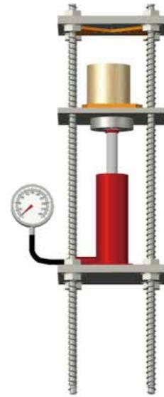
Figure 5: Longitudinal shear test
