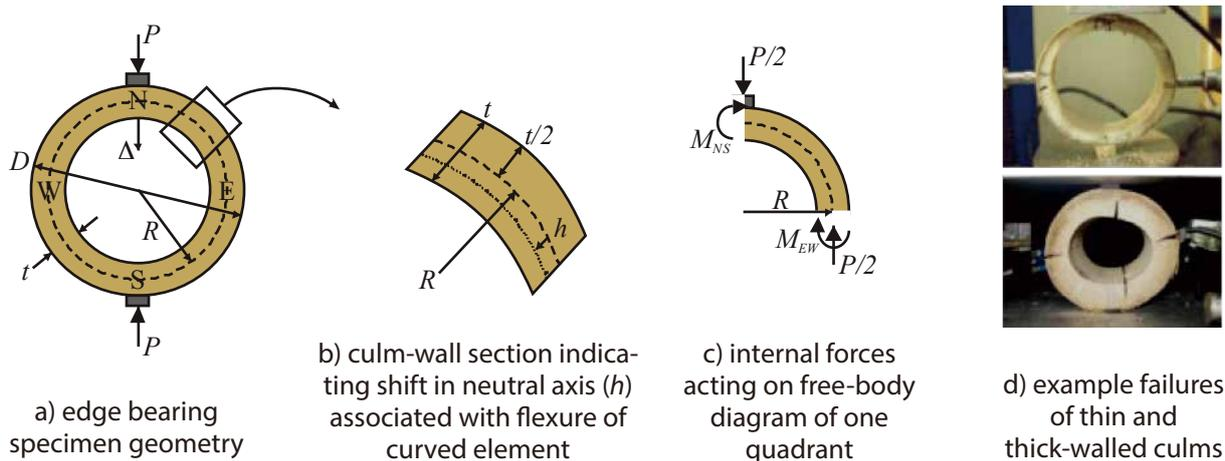
**Figure 7: Edge bearing test specimen geometry and internal reactions.**
