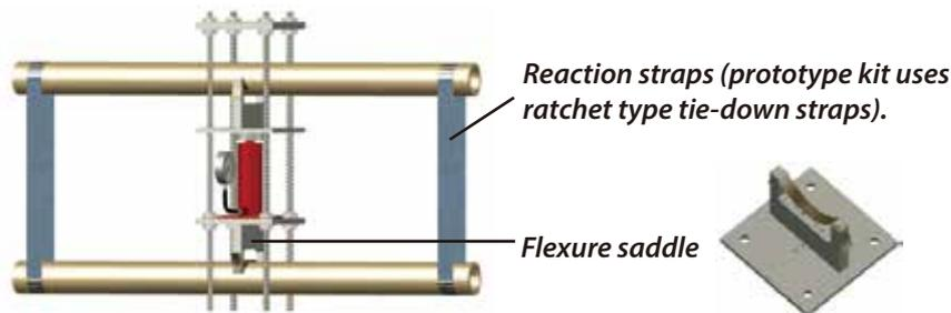
**Figure 8: Full-culm flexure test**
