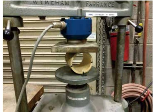
**Figure 10: Mechanical test frame set up for edge bearing test**
