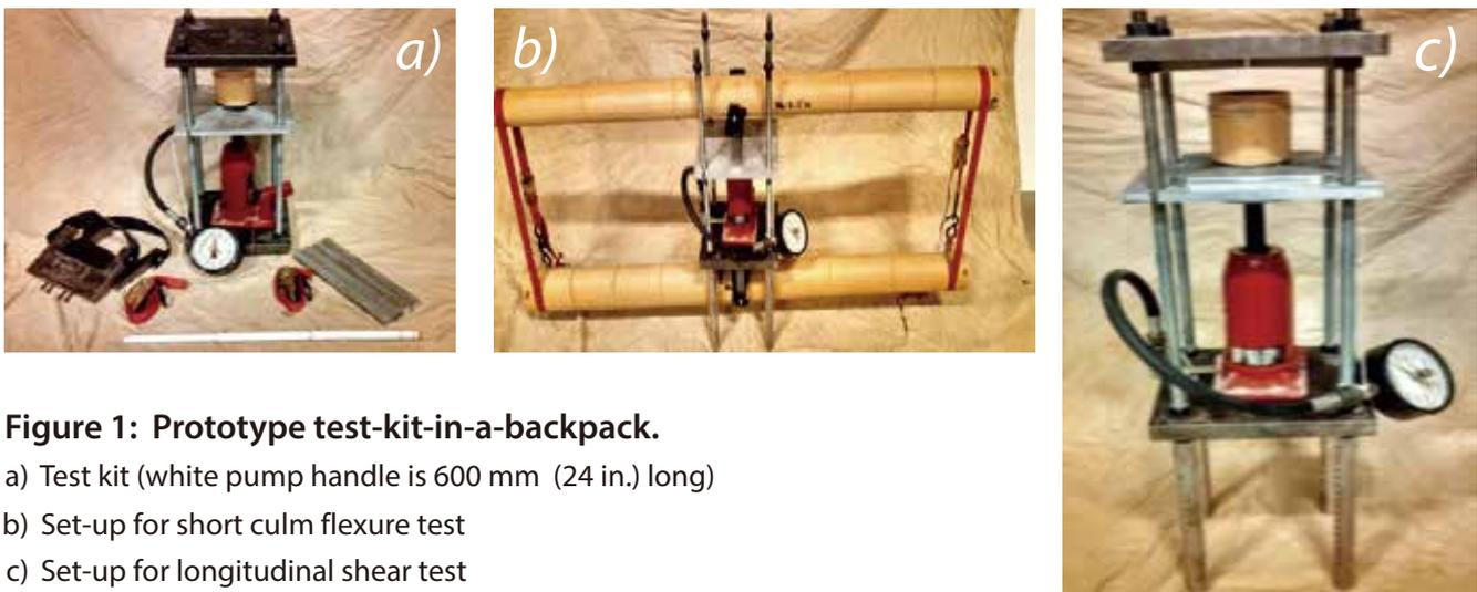
**Figure 1: Prototype test-kit-in-a-backpack.**
