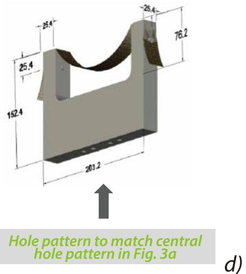
Hole pattern to match central hole pattern in Fig. 3a
