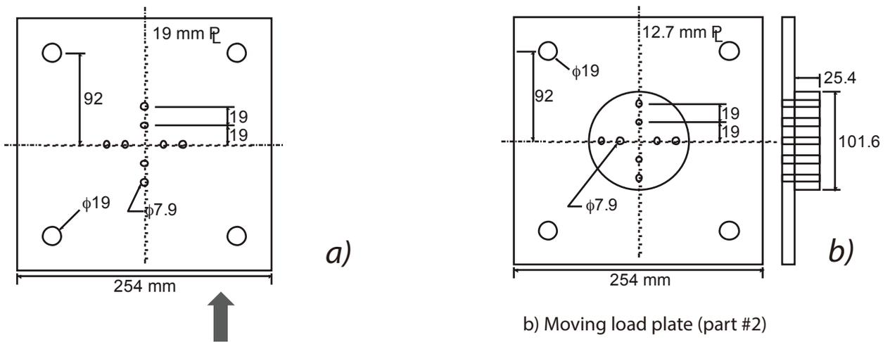
Central hole pattern to match hydraulic cylinder base plate
