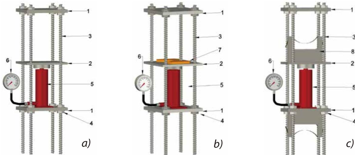
a) Assembly for compression and edge bearing tests
