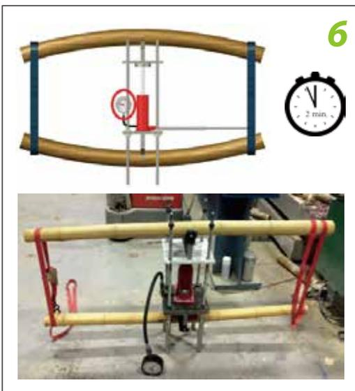
1. Cut specimen length to the desired length  $L$ . To be consistent with ISO 22157,  $L > 20D$  although this is not a requirement provided test results are only compared with other results using the same  $L/D$  ratio.
