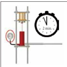
1. Cut specimen length such that  $L = D$ . Specimen ends should be smooth, parallel and at right angles to culm axis. Specimens should not include nodes. Specimens containing nodes are expected to exhibit higher capacities.
