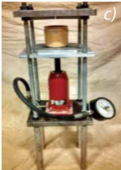
The 'kit' (Figure 1), intended for rapid in-the-field assessment of bamboo mechanical and material properties, is designed to be an inexpensive, robust, portable test apparatus that may be carried, assembled, operated and maintained by a single technician. Presently the kit supports:
