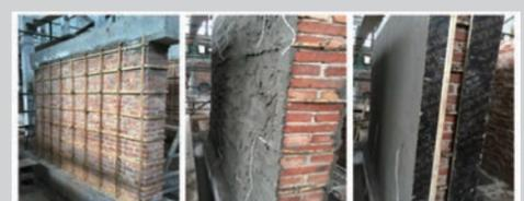
Masonry wall strengthened with bamboo-meshed cement mortar
