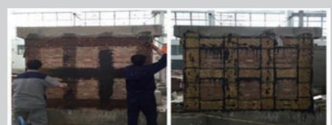
Masonry wall strengthened with bamboo sheets
