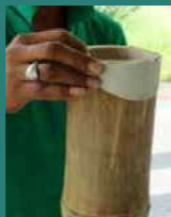
2 Using PVC Mold to Trace
