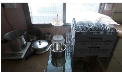
Common 12L pressure cooker for autoclaving media bottles
