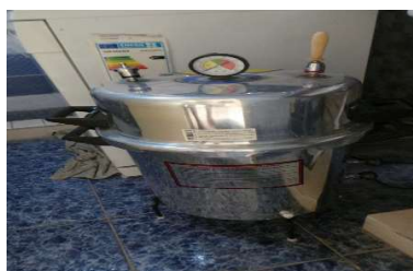
Larger 29L pressure cooker type autoclave
