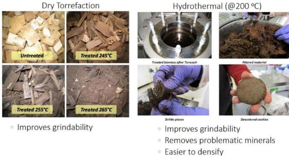
**Figure 19.** Torrefied and wet torrefied bamboo (Daza Montaño et al., 2013).
